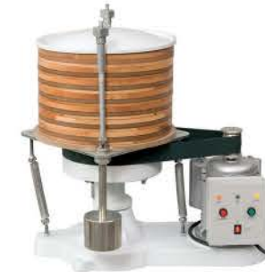
CIRCULAR SHAKING LABORATORY SIEVE DAİRESEL SALLAMALI LABORATUVAR ELEK
